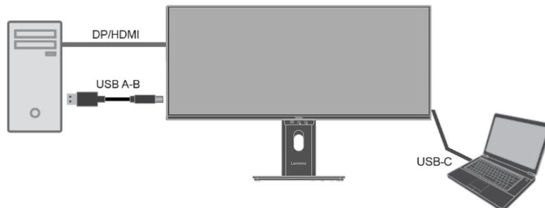
Step 2 The shortcut key of KVM on right direction of five-way key. The USB devices will be switched to another upstream port after OSD disappears. Note: KVM operation may cause USB device to be interrupted.
