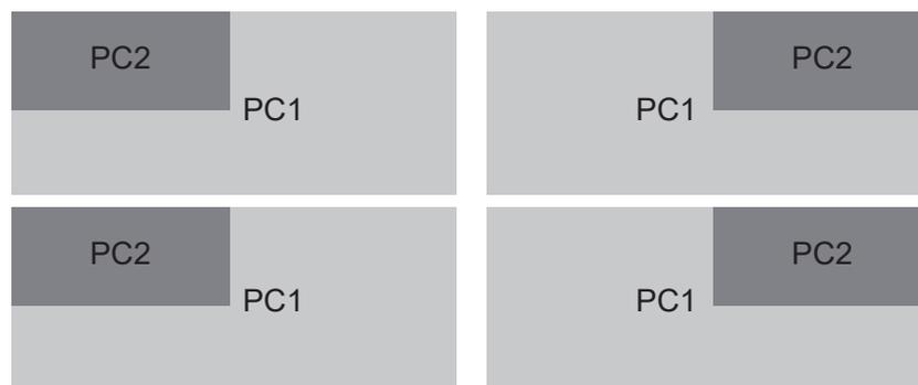
As same to PbP, the PiP (Picture-in-Picture) function can receive two different video sources too. The best resolution of foreground PC2 is 3440x1440@60Hz, maximum resolution is 3440x1440@100Hz. The foreground PC2 sub-screen can be placed on top left, top right, bottom left, bottom right of monitor.
