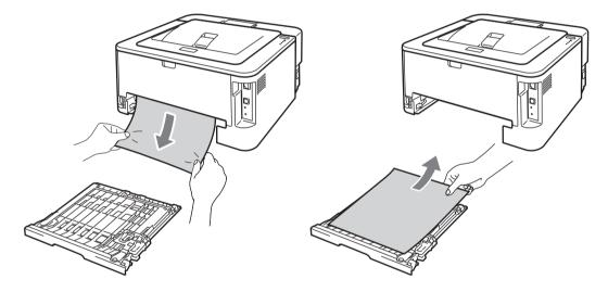
12 Make sure that the jammed paper does not remain under the machine from static electricity.
