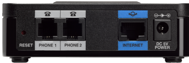
Figure 2. Ports on Cisco SPA112 ATA 2 Port Adapter
