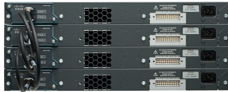
Figure 2. FlexStack Stacking on 2960-S and 2960-SF Switches
