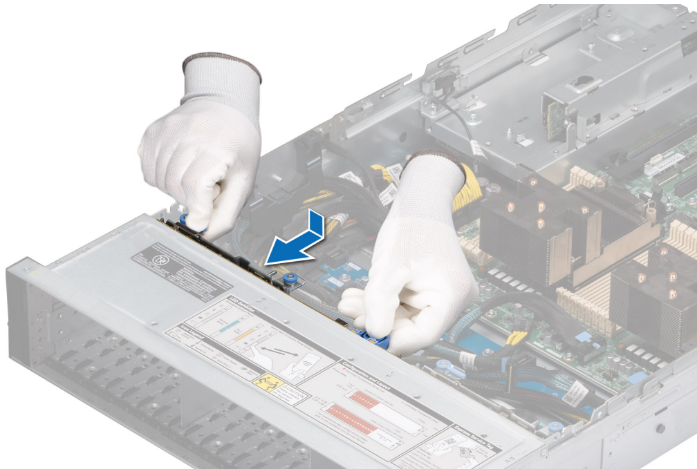
Figure 50. Installing the drive backplane
