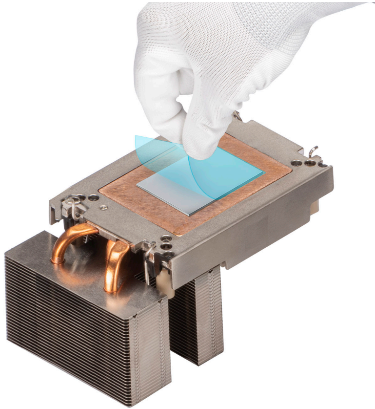
Figure 73. Remove the Thermal Interface Material (TIM) protective film
