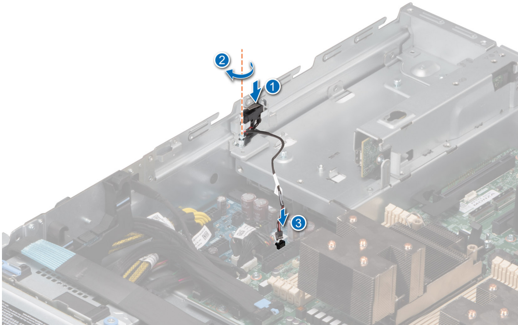
Figure 36. Installing the intrusion switch
