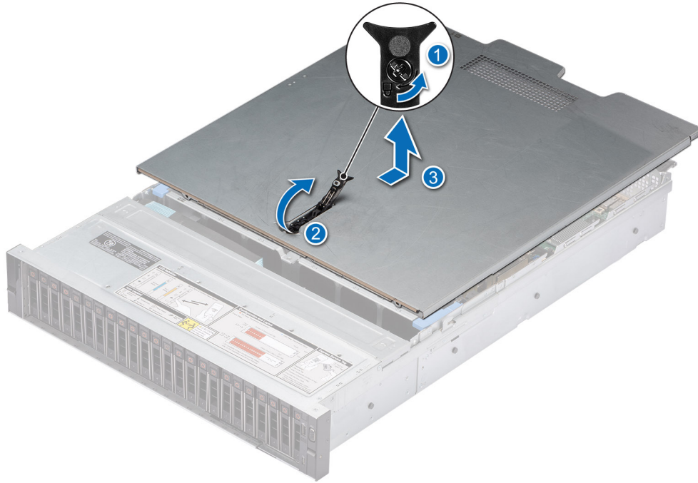
Figure 19. Removing the system cover
