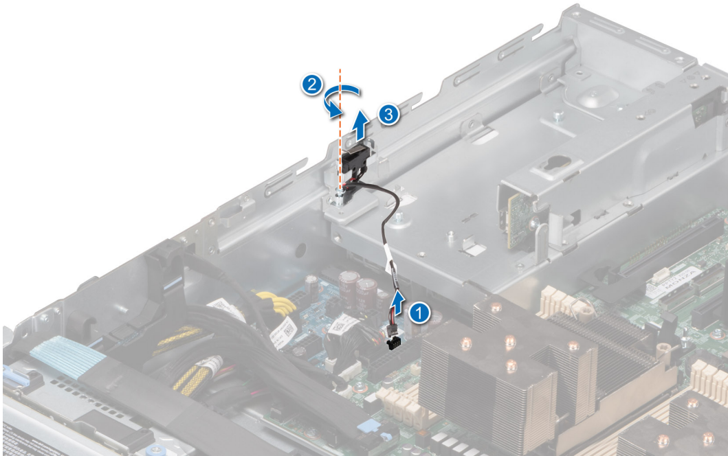
Figure 35. Removing the intrusion switch module
